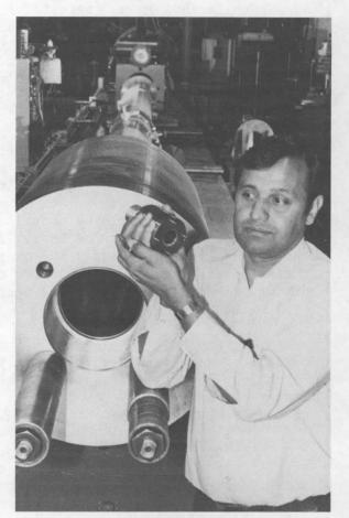
AT THE BREECH end of the Hypervelocity Launcher (HVL), Lalit Chhabildas (1543) holds a barrel extender. The barrel extender is an easily replaceable part of the HVL that holds the aluminum flier plate and receives much of the wear caused by operations.
